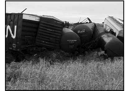
West end of derailment. CN boxcars' coupler is broken off. – Photo © Chip Sherman
